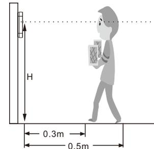
The recommended installation height (H) is 1.45m. It can be adjusted according to the actual scene.
